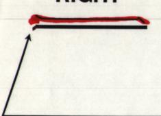
MACHINE OR GRIND STRAIGHT ACROSS - DO NOT NOTCH IN!
